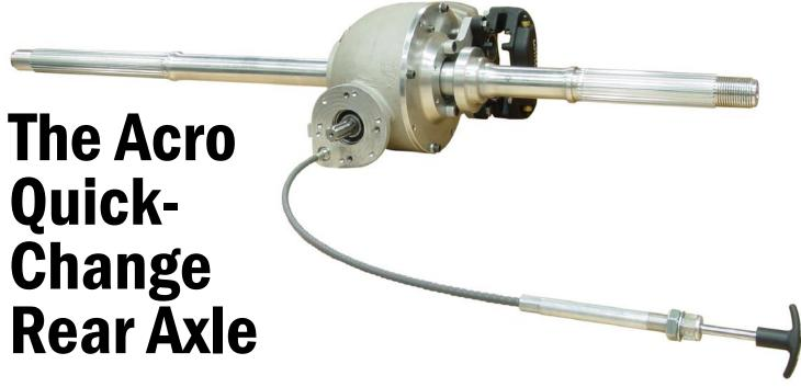
The Acro quick-change rear end is designed with an open axle shaft of either high-strength aluminum or heat-treated steel. This axle is driven by a ring and pinion gear set mounted in a cast aluminum housing. The back section contains the quick-change gears. The housing may be located anywhere along the axle between the chassis carrier bearings according to your installation requirements.
